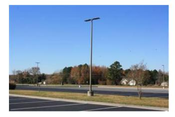
This study assumes replacement of the light fixtures every 15 to 20 years, and pole replacement every 30 to 40 years. When the light poles are replaced, we assume that the underground wiring will also be replaced.
